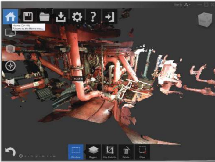
Above: Scan data of cooler inlet pipework imported directly into Autodesk Recap. Right: Screen shot from Navisworks Simulate. Using Navisworks Simulate SCE can save an AutoCAD model to a format that can be read by Navisworks Freedom which is a free 3D viewer.
