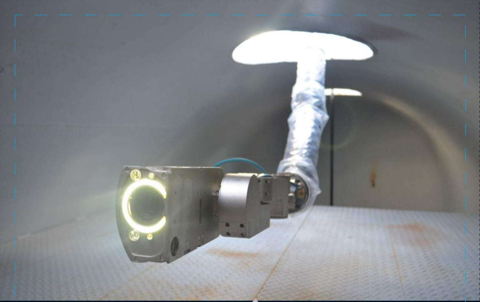
Above and left, the P100 robot “snake arm” robot is due to be trialed in the North Sea this year, as part of efforts to make pressure vessel inspection more efficient.
