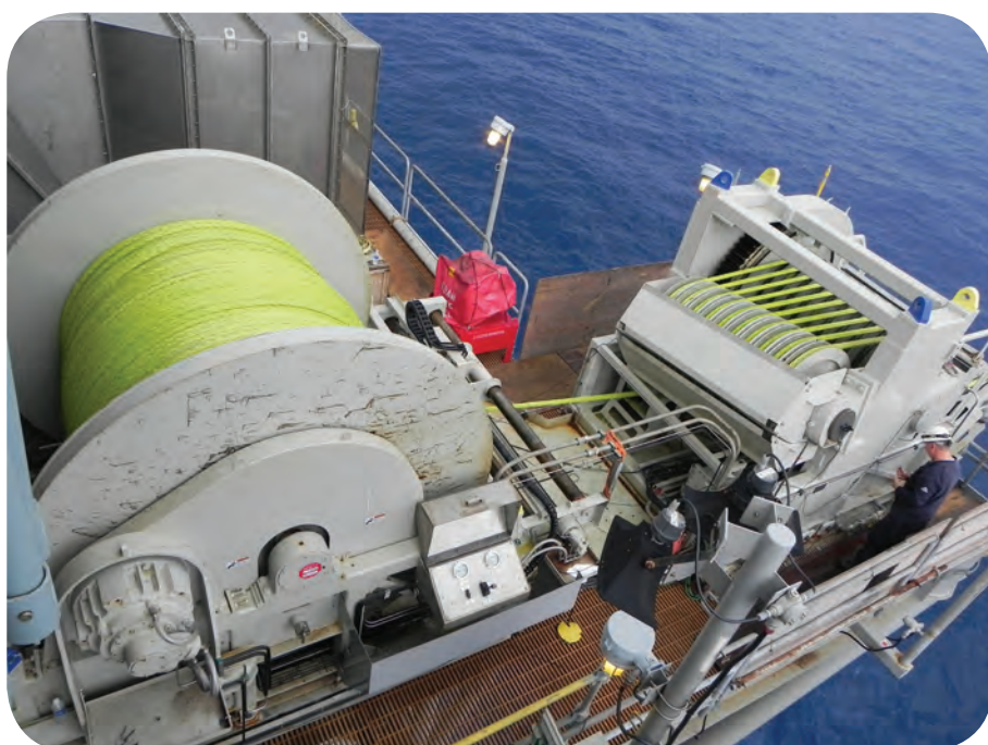
Fig. 3. Lightweight, synthetic rope allowed use of a simple, traction-style winch to meet weight and space restrictions on a cantilevered deck.
