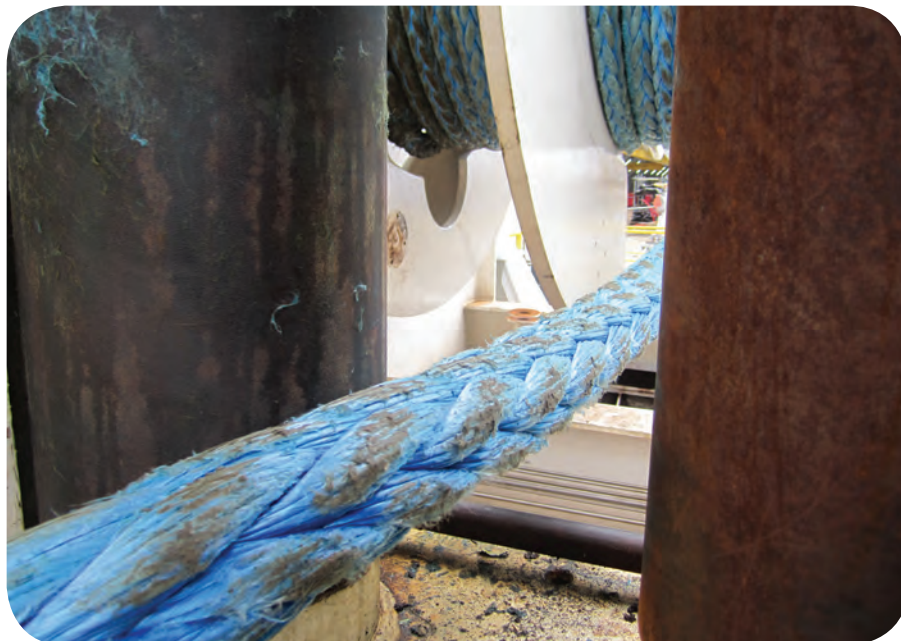
Fig. 6. Abrasion concerns were overcome by making the rope jacket from abrasion-resistant polyester.
